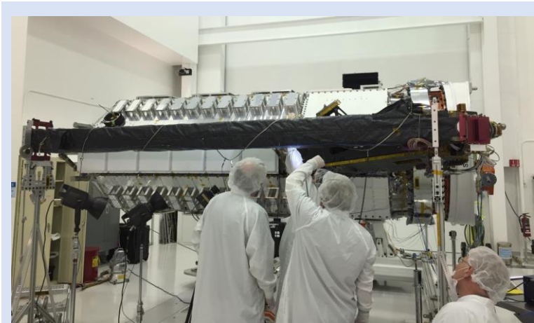
Lower Boom is Integrated, Completed Successful Flight-Like Deployment
