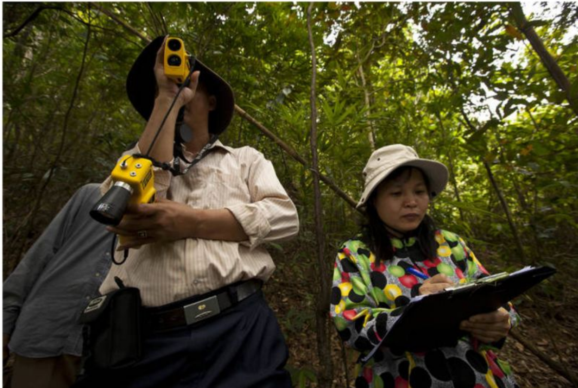
Forest researchers in Viet Nam use laser technologies to measure tree height and thickness.
